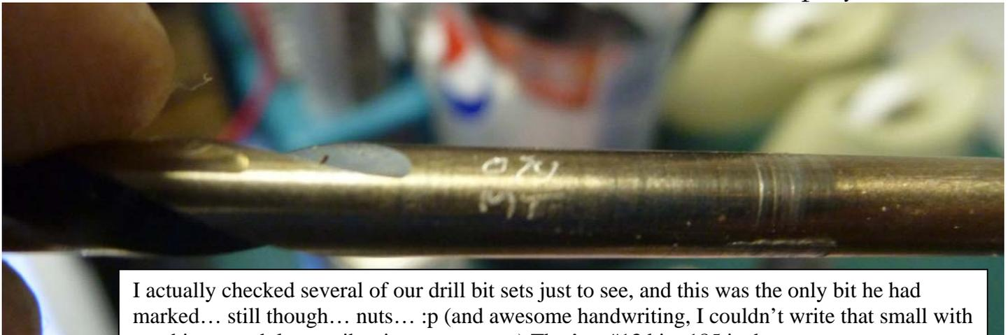
I actually checked several of our drill bit sets just to see, and this was the only bit he had marked... still though... nuts... :p (and awesome handwriting, I couldn’t write that small with anything, much less a vibrating engraver...) That’s a #13 bit, .185 inches across
