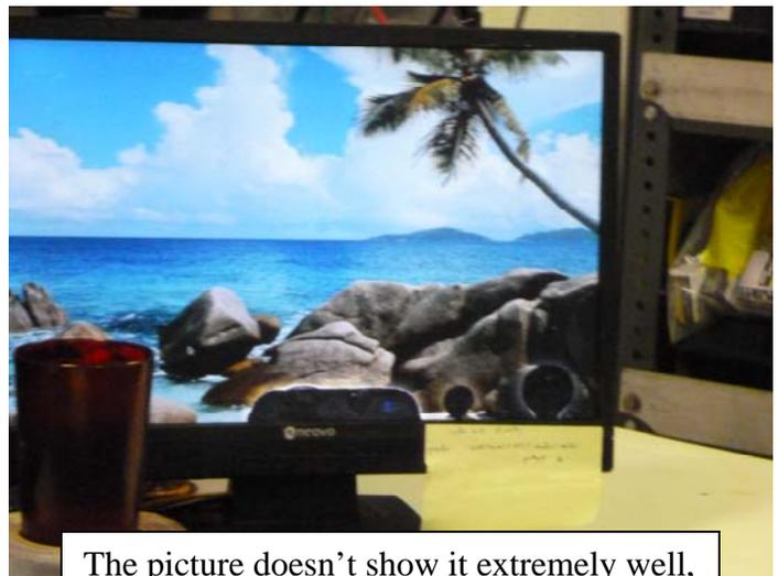
The picture doesn't show it extremely well, but the black splorches coming up from the bottom of the screen are what happens when water gets into the lcd ☹️
