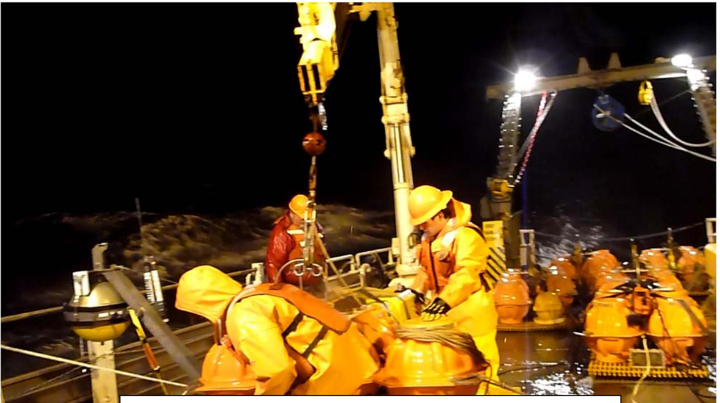
The gadget between the crane hook and the top of the OBS is a quick release that lets us pop the OBS off of the crane once the taglines are clear.
